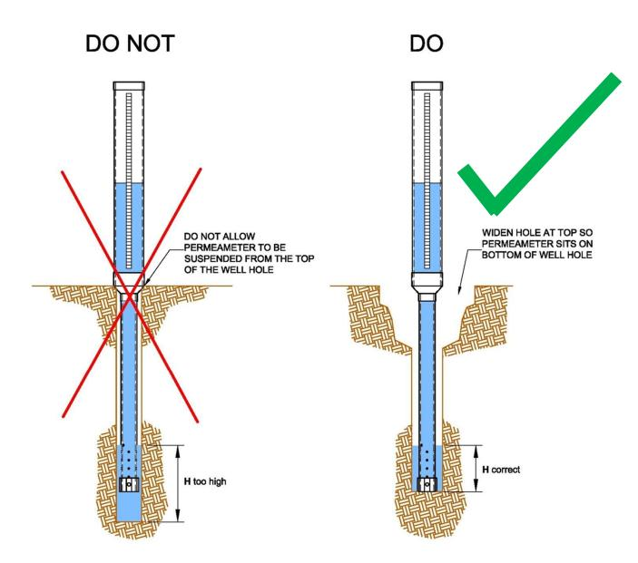
Ensure permeameter is not hanging from the top of the well hole, otherwise H will be incorrect.
